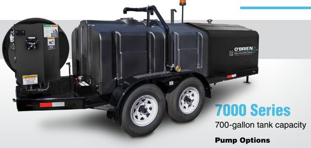
18 GPM at 4,000 psi 40 GPM at 2,000 psi 40 GPM at 3,000 psi
